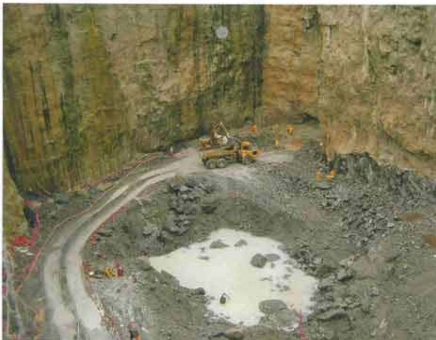
Mining the Koidu kimberlite pipe in Sierra Leone – this is one of Shaft Sinker's more unusual contracts, combining elements of both shaft sinking and open pit mining (photo: Shaft Sinker).
